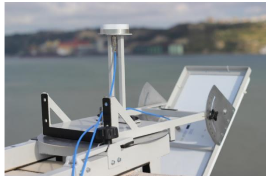
Figure4– Upward and Downward looking antennas of the SARGO system
