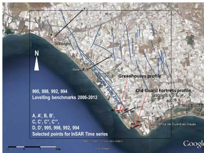
Figura 3 – Faults distribution over Goggle Earth in the area of study. Red lines represent levelling profiles for the period 2006-2012. (Galindo-Zaldívar *et al.*, 2013). Black lines connect points from which their MTI-InSAR mean LOS velocities time-series have been retrieved. These points are depicted by triangles.
